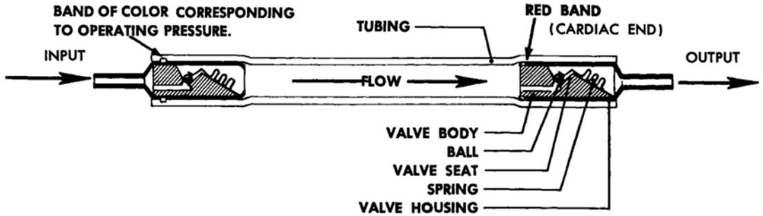
FIG. 1. Schematic drawing of valve mechanism.
