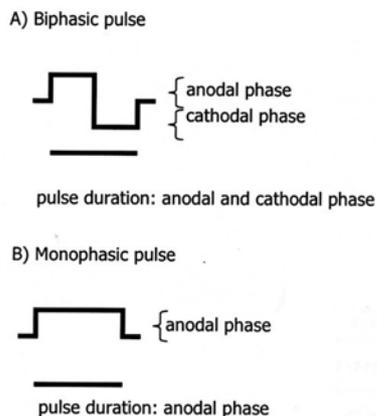
Fig. 1. Schematic of monophasic and biphasic pulse forms.
